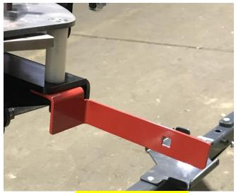
4) Next, place part number 120100584 on the inside of the large mounting bracket as shown below and use the following hardware numbers HDW2050 & HDW2020 to fasten the mounting bracket to the mating part.
